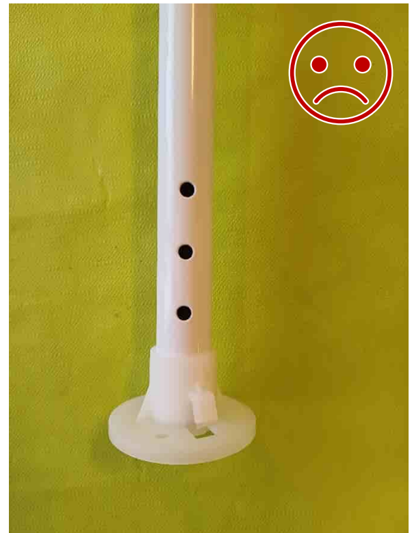
Figure 14 WRONG . Consumer structure. The support leg is plastic, not locked to the pole, and cannot withstand stress.
