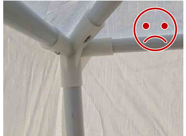
Figure 13 WRONG . Consumer structure. The pipes do not lock into the joint.
