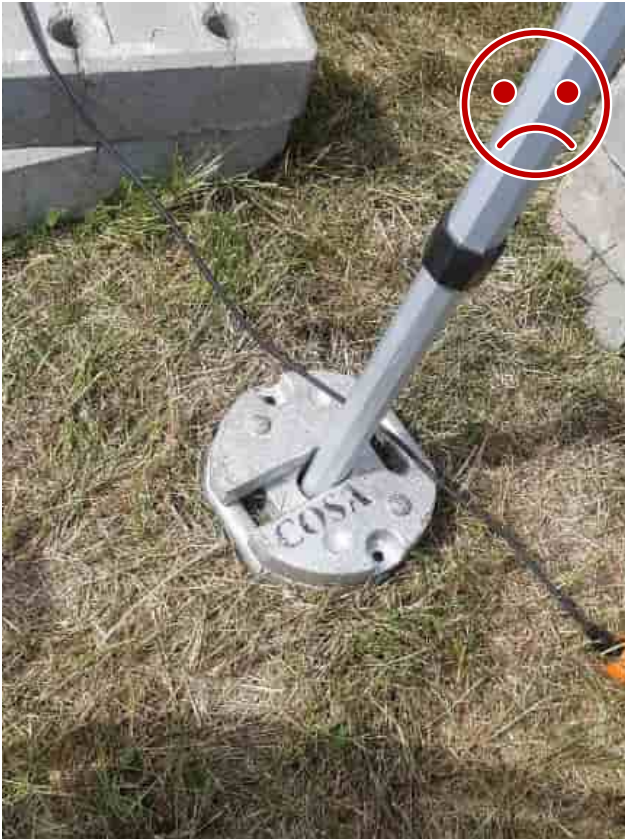
Figure 1 WRONG. The weights are not interlocked. Gravity will cause the weights to come loose, and they will not secure the pole while the wind shakes the tent.
