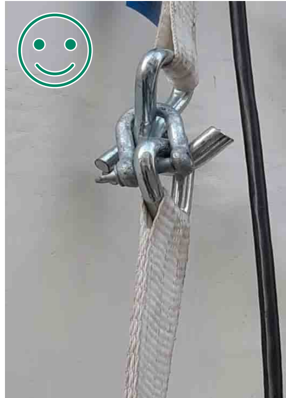
Figure 8 RIGHT. Hooks locked with a shackle.
