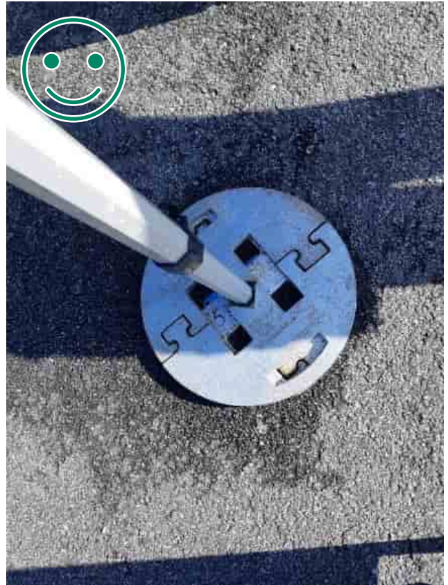
Figure 4 RIGHT. Two layers of weights in opposing directions lock the layers around the pole when a sufficiently large, solid bottom plate is used. The feet of a corner pole must be able to withstand this weight.
