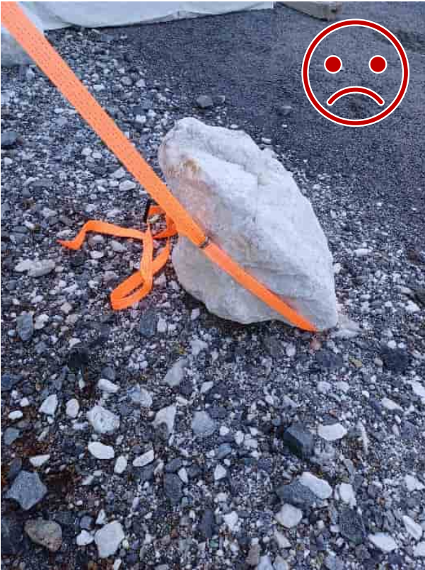
Figure 5 WRONG. The strap is not locked to the stone, which also features sharp edges.
